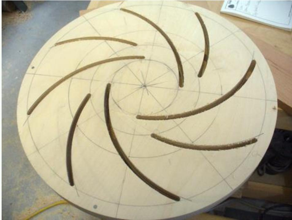
At this point we put it back on the lathe and with a 1/4" drill bit in a Jacob`s chuck on the tailstock we drilled a hole completely through the center. We also drilled a couple of holes around the very outside edge so that we could use tommy bars to tighten.
