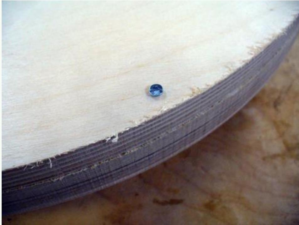
Next, we attached a faceplate to the center of one of the disks using screws that **just went only into this one!** The faceplate will be permanent so you need to get one specifically for the Longworth chuck. Once the faceplate is attached to the disks put it on your lathe and turn the disks perfectly round, removing as little wood as possible to maximize the size of the chuck.
