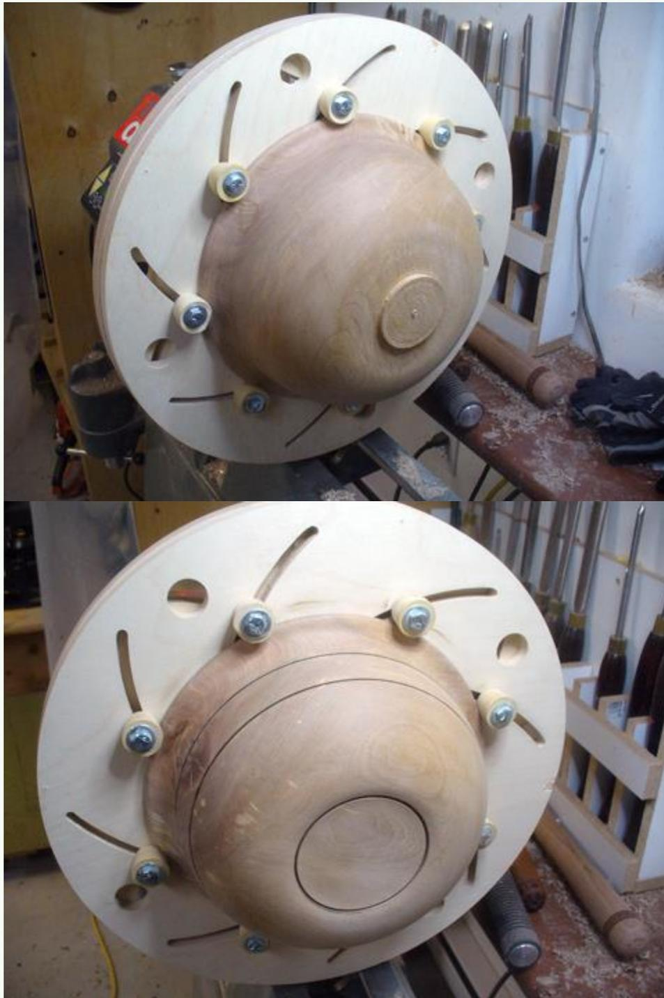
Because there are 4 arcs that don't come as close to the center as the other 4 there is a limit to how small of a piece you can fit on. The solution is to remove those 4 bolt assemblies and just use it with the 4 buttons on the larger arcs. This isn't a problem since a smaller piece will require less holding power. Another solution is to just make a smaller one with just 4 buttons.
